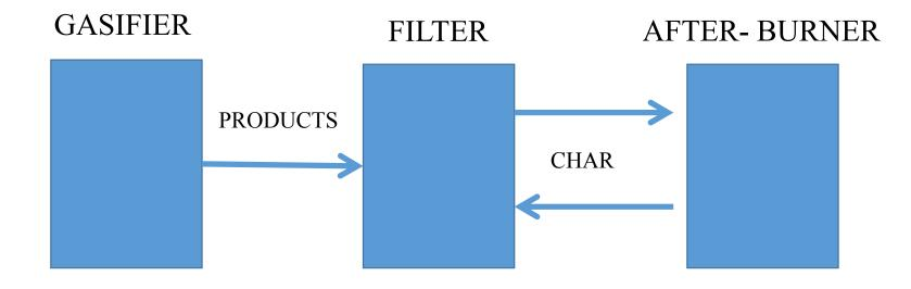
Char reacts on a secondary stage with air at an elevated temperature (450 °C – 750 °C). The scope is the distribution of heavy metals between the gaseous and the solid phase. Usually a reduction > 20 % is sufficient for reduction into accepted environmental limits.
