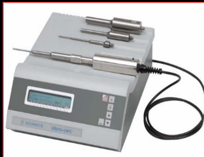
130 W, 20 kHz VCX-130 Sonics and Materials (Danbury, CT, USA) with Ti-Al-V probe (13 mm)
