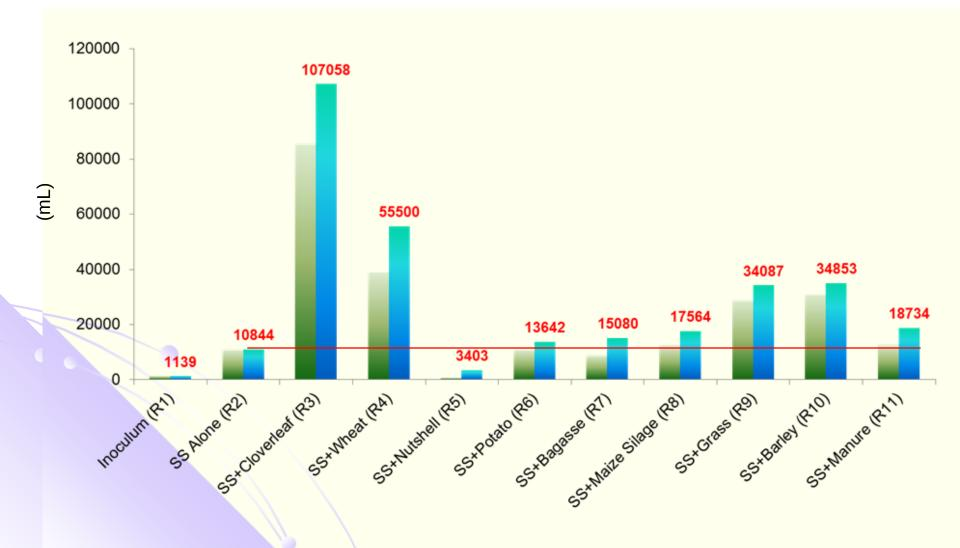
Biogas Production for Single Substrate Digestion
