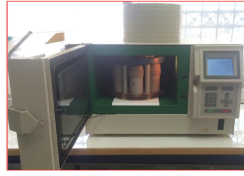
Microwave system (MultiwaveB30MC030A) (Anton Paar, Austria)
