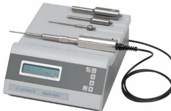
130 W, 20 kHz VCX-130 Sonics and Materials (Danbury, CT, USA)  $\mu\text{e}$  Ti-Al-V probe (13 mm)
