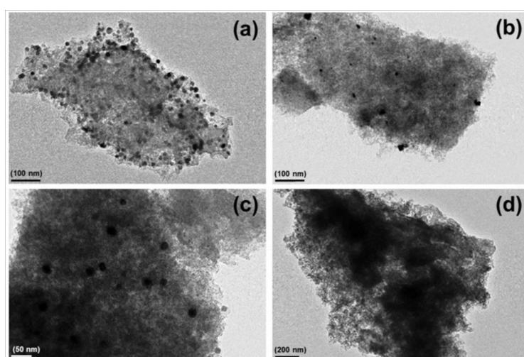
Ni, Cu, Pt, Pd on micro/mesoporous carbon
