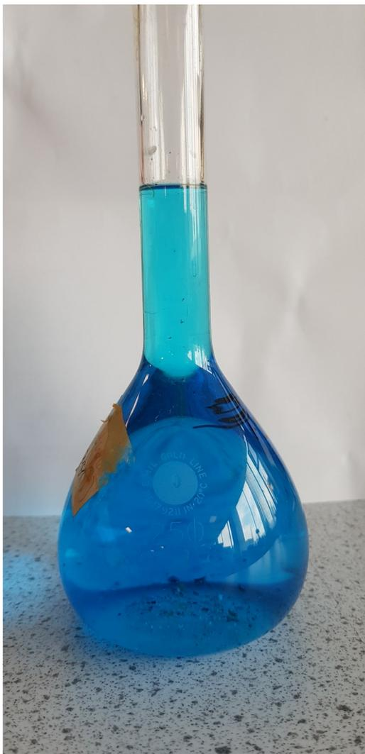
Figure 3. Samples digested in 50/50 nitric acid/water
