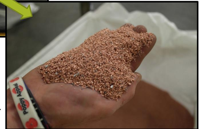
Figure 1. Cables in their raw form (top), cables after shredder (middle), copper from cables in final form (bottom)
