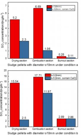
SO<sub>2</sub> concentration at three sections with/without CaO Addition of CaO (1%) in sludge pellets can reduce the average  $SO_2$ concentration in each
