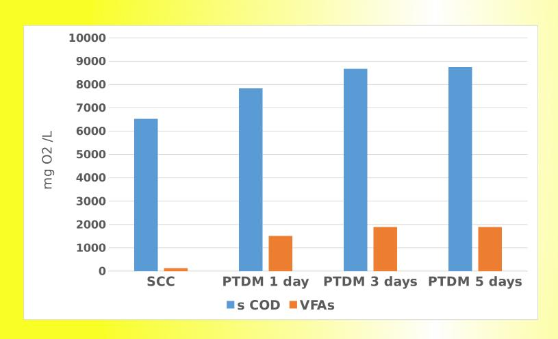
Figure shows how the 1 day - HRT contributed to an important optimization of sCOD and VFA concentrations compared to the SCC test, with an increasing of more than the 15% and 55%, respectively. Anyway, longer HRT of 3 days brought to further sCOD and VFA productions' increasing at 25% and 65%, respectively. Instead, a HRT of 5 days did not lead to better performances.
