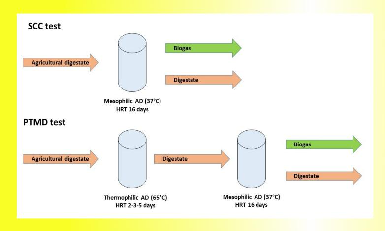
The performances of the PTMD were evaluated in semi-continuous mode too and compared with a semi-continuous control test (SCC). Figure 2 summarizes the SCC and PTMD processes. In the PTMD test the mesophilic digestate was digested at 70°C and then digested for a second time at mesophilic temperature (37°C). On the contrary SCC was simply digested a second time at 37°C.
