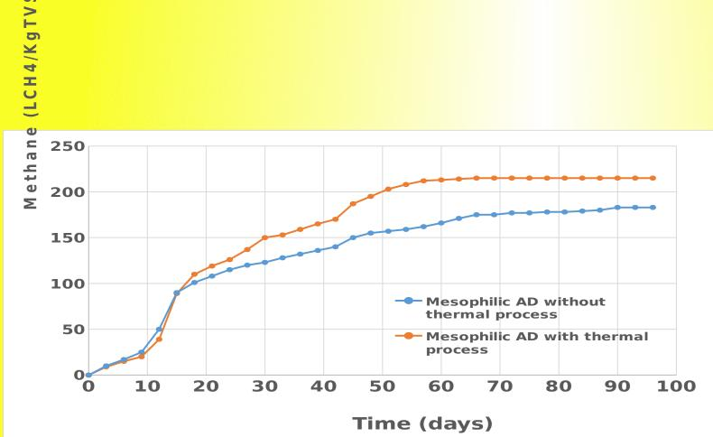
The trend of the BMP tests, having similar exponential growth in the first 15 days, demonstrate that thermal treatment seems to be efficacy on the degradation of more recalcitrant and degradable slowly organic compounds. The kinetic of residual simple compounds (sugars and carbohydrates) was not affected by thermal treatment. Instead, it improved the solubilization of more complex molecules, such as lipids and proteins, present in high concentration in digestate from manure AD.
