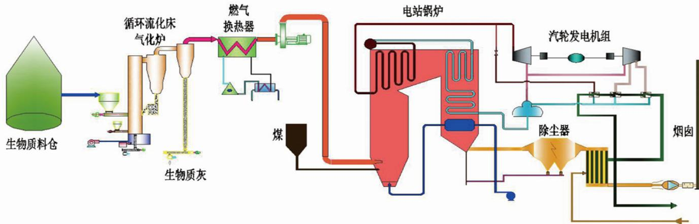
**Biomass gasifier + Coal-fired power plant**
