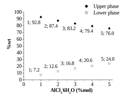
With the increase of the catalyst, the reaction became fast and the bottom aqueous phase increased.
