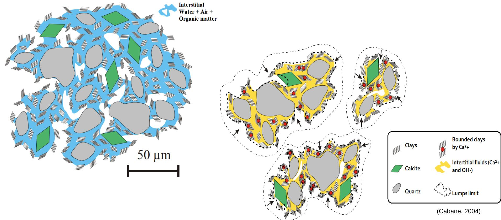
Fig : Approached structure and behavior of sediment materials when blended
