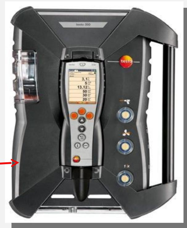
A new model “Testo-350” gas analyzer was used to measure temperature and gas concentrations ( $O_2$ ,  $CO$ ,  $C_xH_y$ , and  $NO$ ) at different locations in the conical FBC, as well as at stack.
