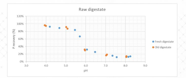
The P recovery generally increases with the reduction of pH value. 90% P is released into the liquid phase with a pH value close to 5.0
