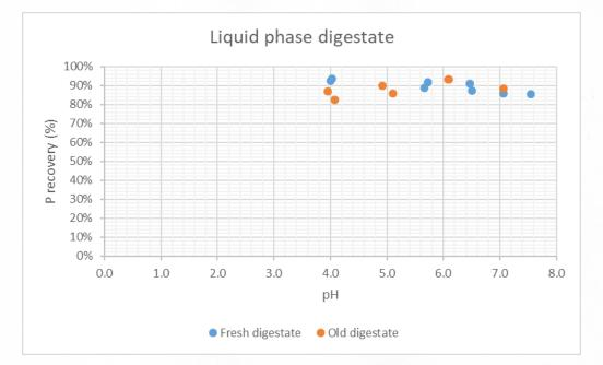
P recovery reached 90%. Although, P concentrations in this stage were lower than the concentrations of the first stage.
