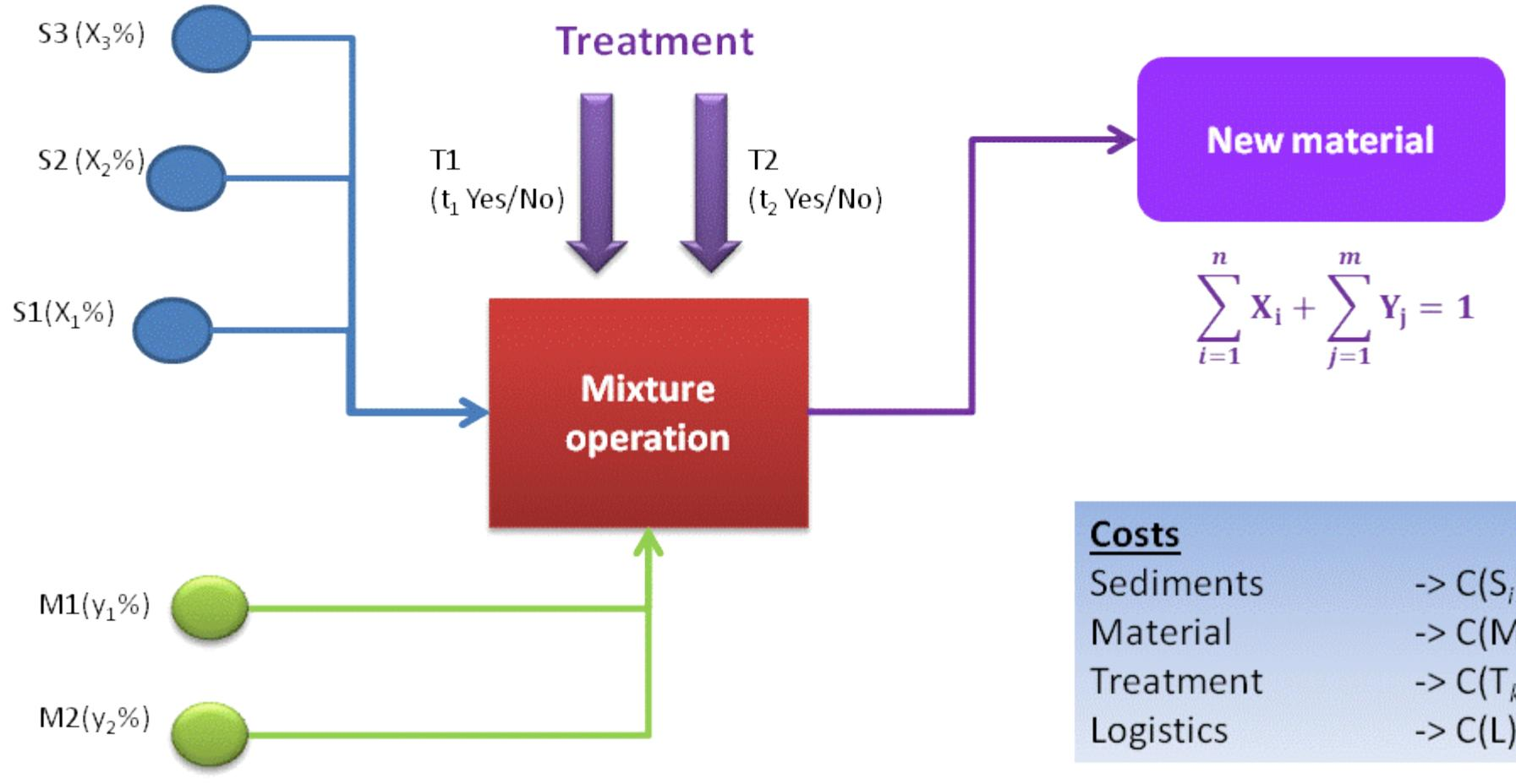
$$\sum_{i=1}^n X_i C(S_i) + \sum_{j=1}^m Y_j C(M_j) + \sum_{k=1}^K T_k C(T_k) + C(L) \rightarrow \text{Min}$$
