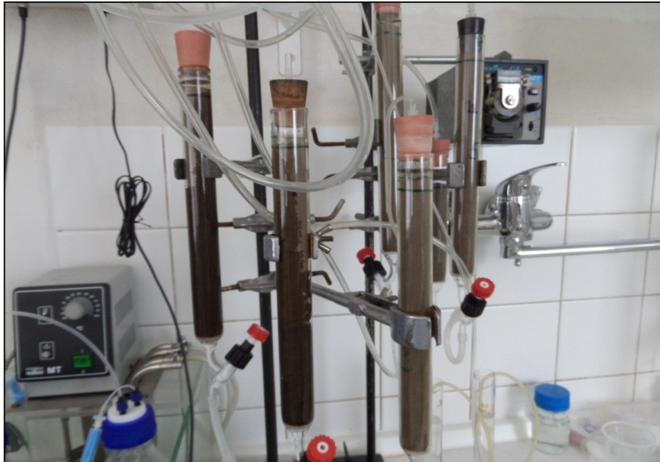
Glass columns filled with contaminated soil
