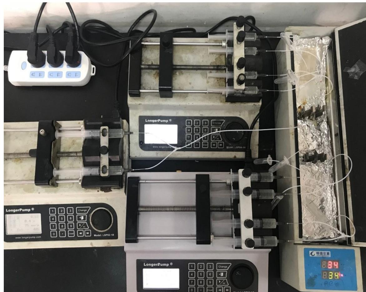
Microfluidic biofilm catalytic system
