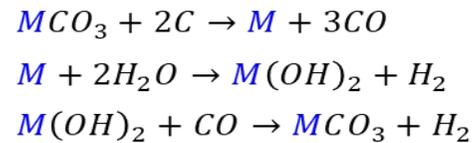
❖ Explaining Boudouard reaction mechanism:
