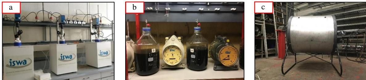
**Fig. 2** a: fermentation reactors in water bath; b: fermentation reactors in acclimatized chamber; c: aerobic tumbler
