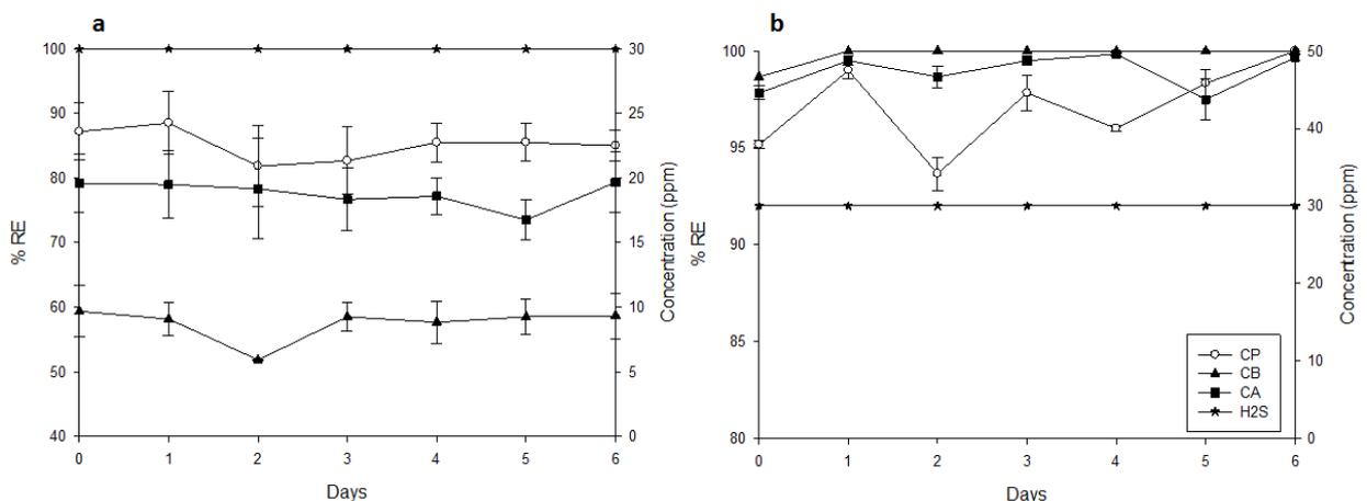
**Fig. 7.** H<sub>2</sub>S removal efficiency at the (a) lower section (height: 0.27 m; retention time: 20 s) and (b) middle section (height: 0.54 m; retention time: 40s) of biofilters filled with different compost mixtures. H<sub>2</sub>S inlet concentration: 30 ppm. CA, manure + rice husk; CP, manure + pruning waste; and CB, manure + sugarcane bagasse.
