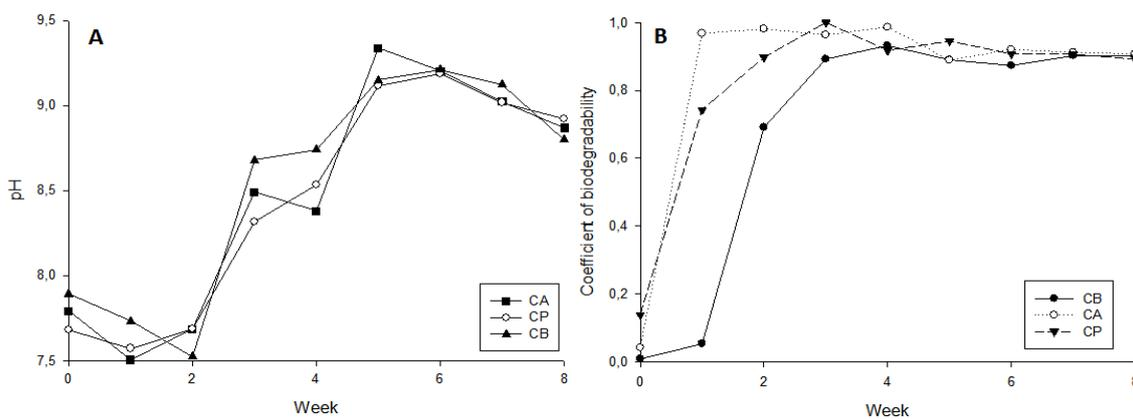
**Fig. 3** Evolution of (a) pH and (b) coefficient of biodegradability of the reactors during the composting processes. CA, manure + rice husk; CP, manure + pruning waste; and CB, manure + sugarcane bagasse.
