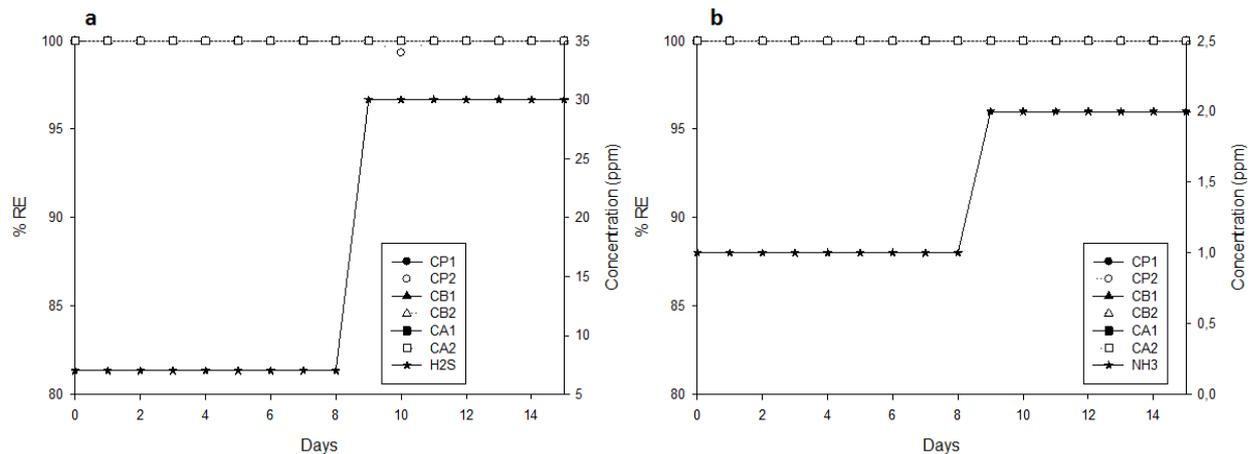
**Fig. 6** Inlet concentration (Retention time 60 s) and removal efficiency of (a) H<sub>2</sub>S and (b) NH<sub>3</sub> in biofilters with different compost mixtures. CA, manure + rice husk; CP, manure + pruning waste; and CB, manure + sugarcane bagasse.
