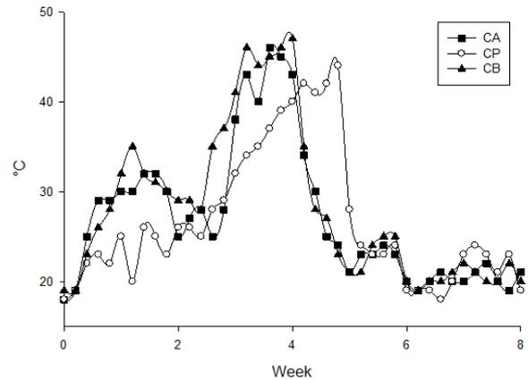
**Fig. 2** Composting thermal profile of manure mixed with rice husk (CA), waste pruning (CP) or sugarcane bagasse (CB).
