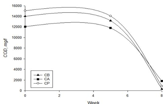
**Fig. 5.** Chemical Oxygen Demand (COD) in the composting processes. CA, manure + rice husk; CP,
