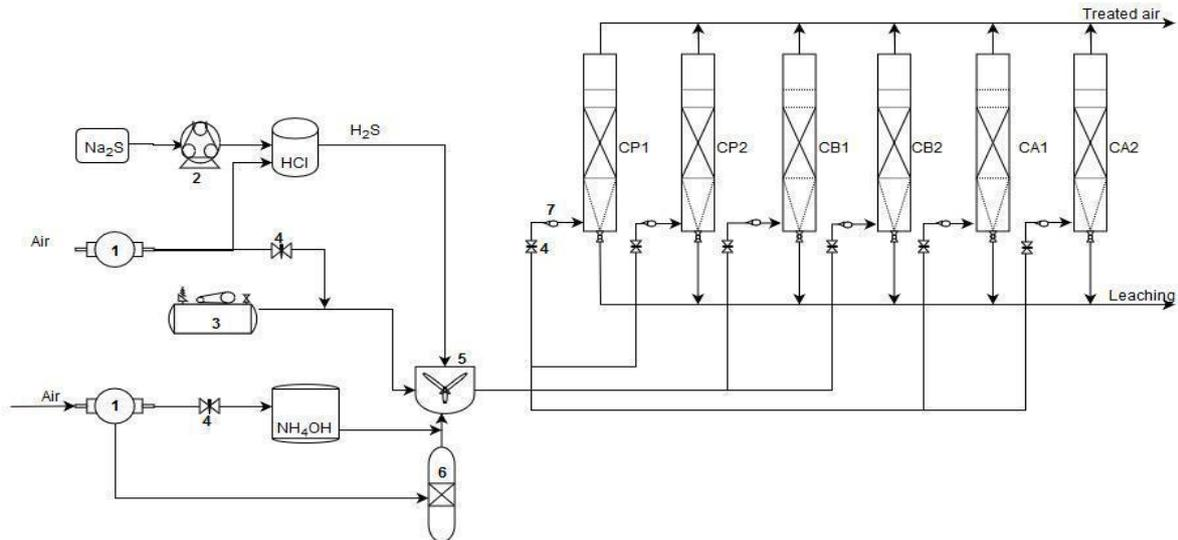
**Fig. 1** Gas generation system and laboratory scale biofilters. 1. Vacuum pump, 2. Peristaltic pump, 3. Air compressor, 4. Valve, 5. Mixing chamber, 6. Humidifier, 7. Manometer, CP. manure + pruning waste, CB. manure + sugarcane bagasse, CA. manure + rice husk (number 1 or 2 indicate replicate biofilter system).
