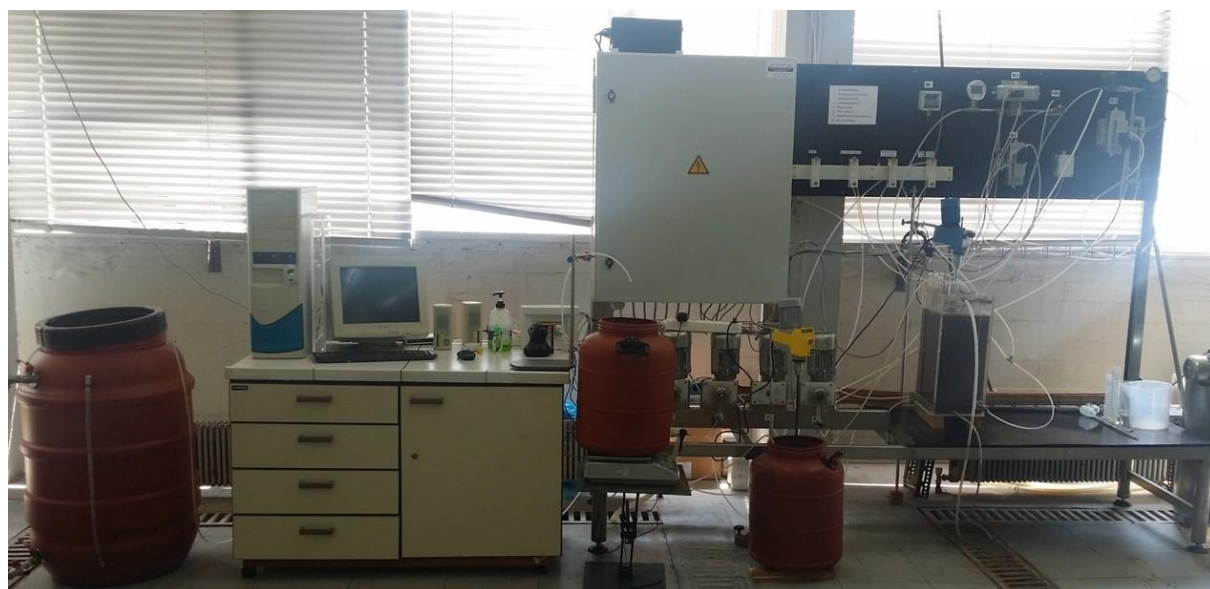
Fig. 1. Pilot-scale MBR system.
