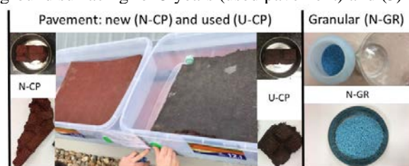
Figure 1. Tested materials for playground surfacing: N-CP, U-CP, N-GR.
