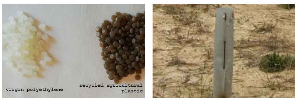
Fig. 1. Pellets of the plastics used (left). An example of tube shelter (right).
