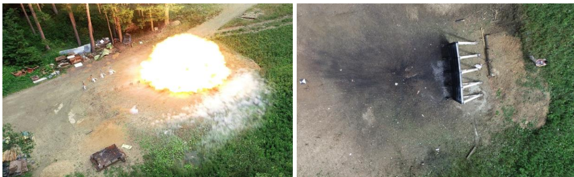
Fig. 5 Photograph of the explosion test (left) and overall state of the construction after the test (right)
