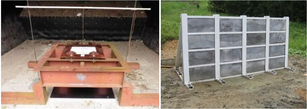
Fig. 3 Configuration of the slab specimen blast test (left), shield system for protection of critical infrastructure (right)
