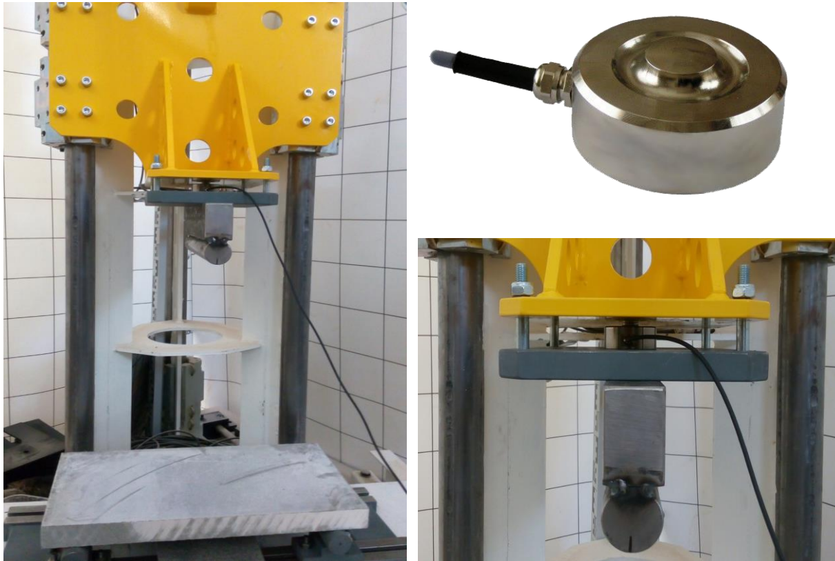
Fig. 2 Drop test device – general view (left), sensor (right above) and placement of the strength sensor (right down)
