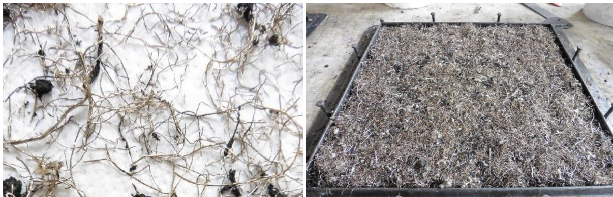
Fig. 1 Waste steel fibres from tires (left), mould with preplaced fibres (right)
