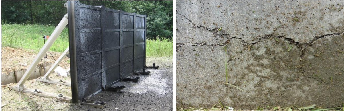
Fig. 6 The shield system after blast test (left), detail of one SIFCON slab (right)
