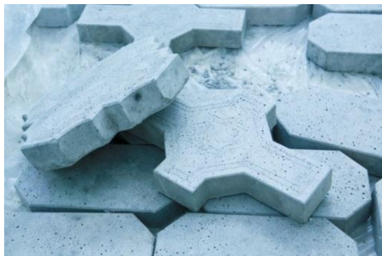
Figure 2. Samples of paving slabs, that for the first time were produced with the use of solids of industrial wastes from titanium-magnesium production
