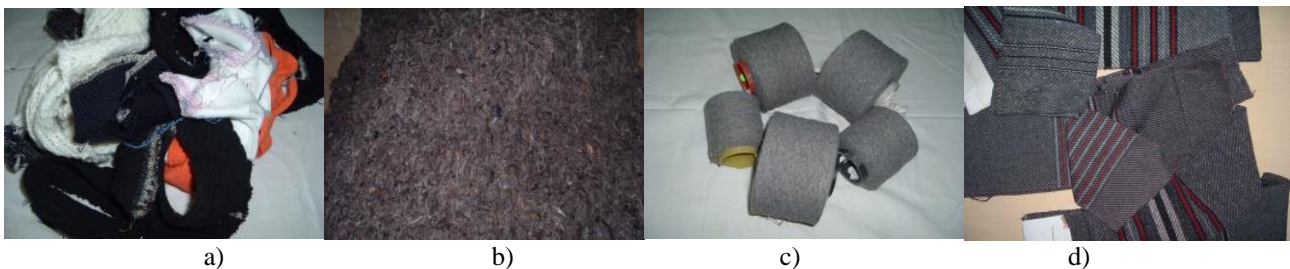
Fig. 1 Characteristic elements of technologic flow: a) textile waste; b) recovered fibers c) open end yarn spun; d) decorative products made of yarn containing recovered fibers
