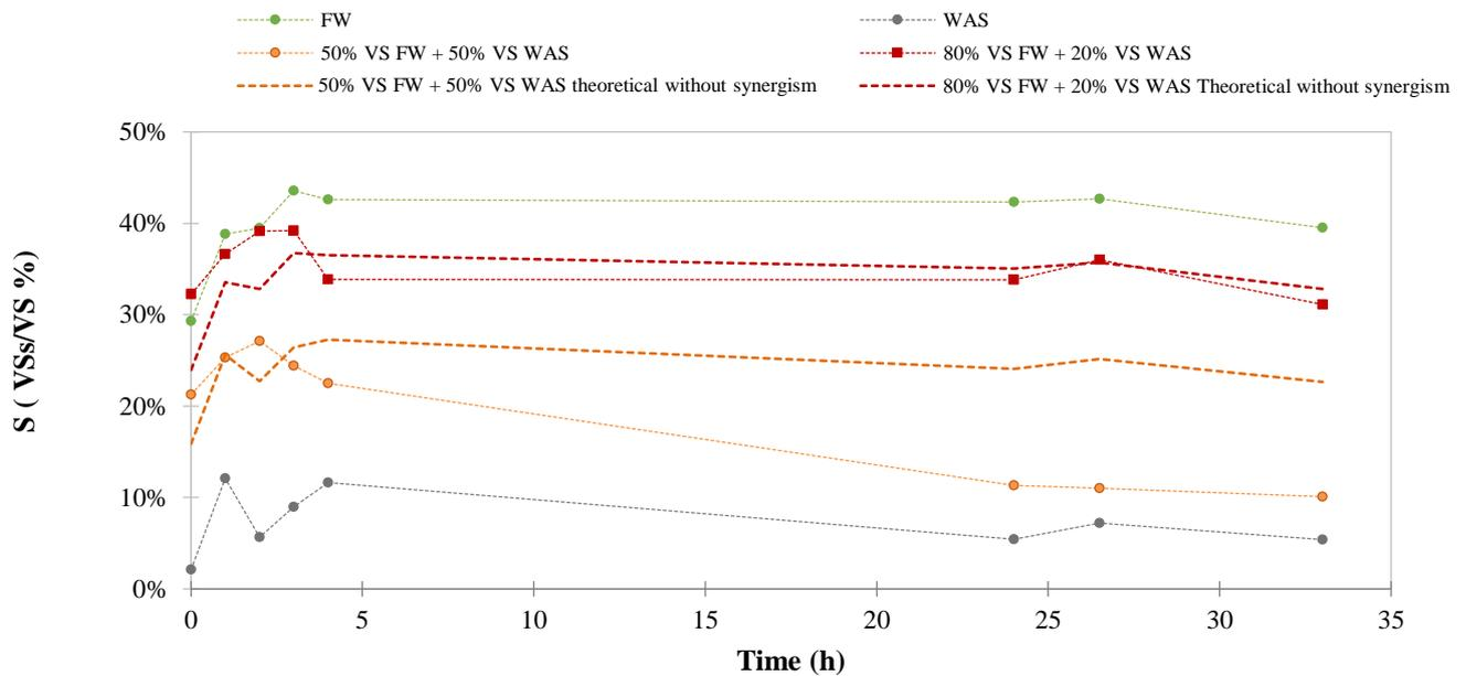
**Fig. 8** Change of solubilisation of FW with WAS under thermal pre-treatment at 55 °C during 4h (discontinuous curves are referred to the expected values of solubilisation if no synergism was observed)
