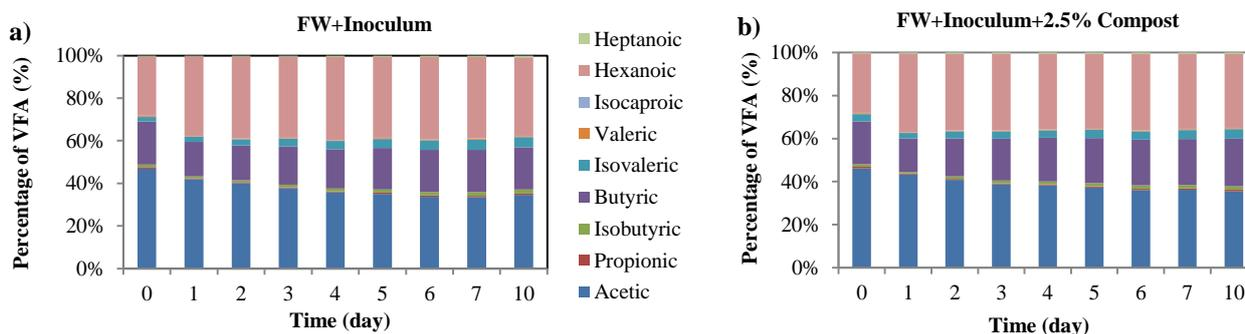
Fig. 2 Individual VFA distribution in batch treating FW with 0% (a) and 2.5% (b) mature compost at pH 6
