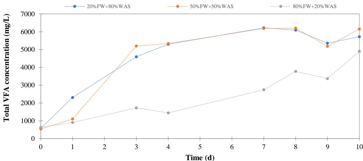
**Fig. 10** Total VFA of discontinuous assay with 2h 30 min pre-treated WAS
