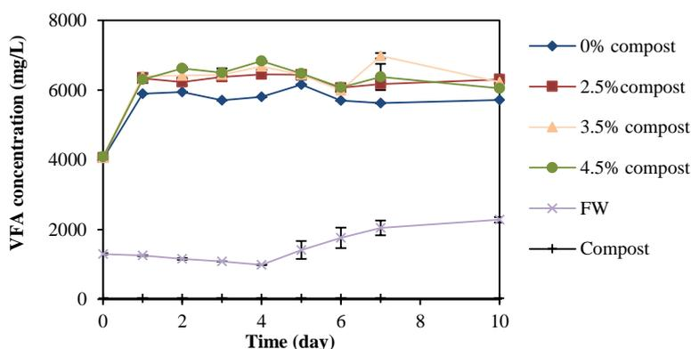
Fig. 1 Progress of VFA production in batch of acidogenic fermentation of FW at 35 °C and pH 6
