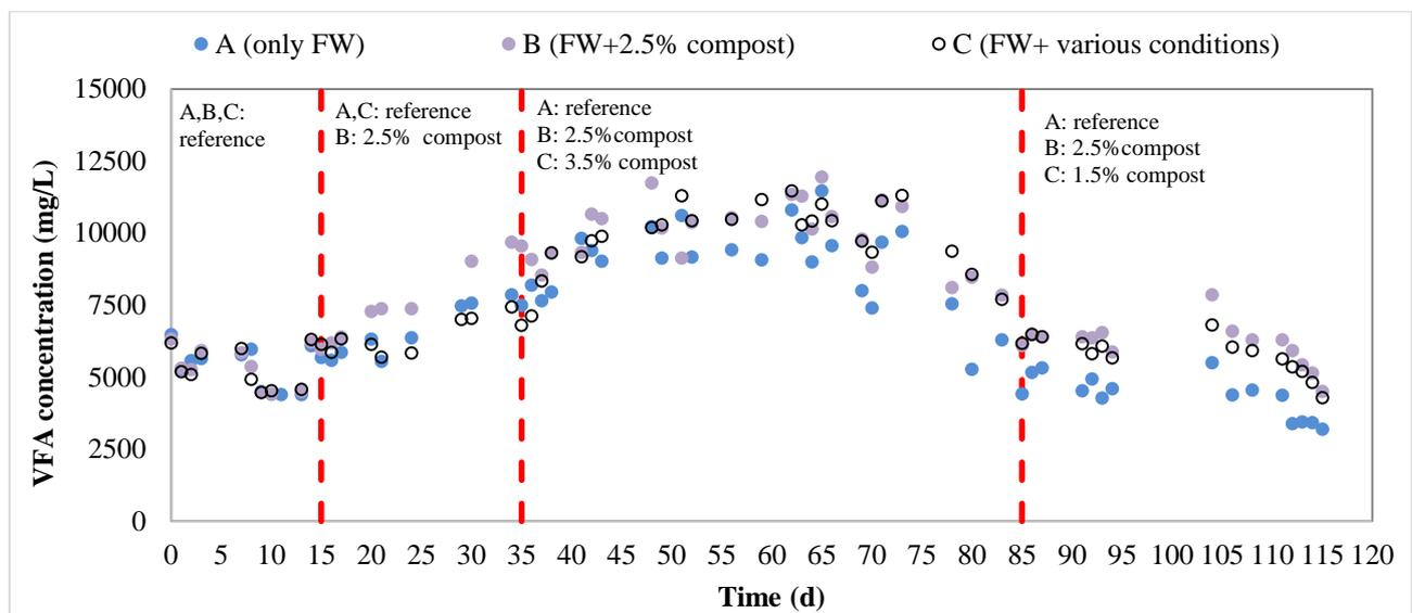
**Fig. 3** VFA concentration in acidogenic fermentation of FW with different percentage of mature compost (temperature 35°C, pH near 6, HRT 3.5 days)
