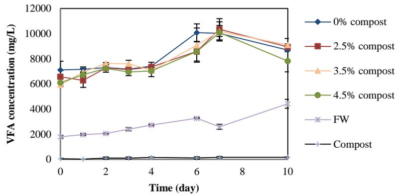
**Fig. 4** Progress of VFA production in batch of acidogenic fermentation of FW at 35 °C and pH 7
