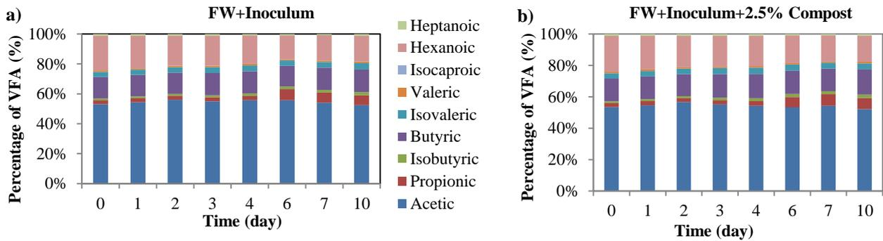
**Fig. 5** Individual VFA distribution in batch treating FW with 0% (a) and 2.5% (b) mature compost at pH 7
