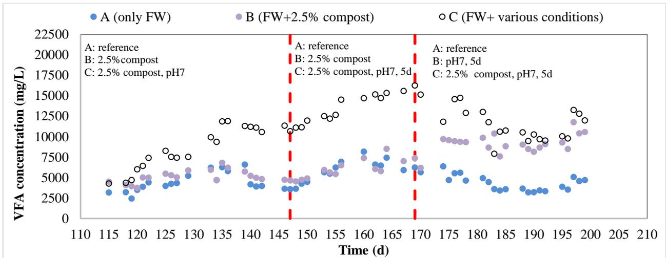
**Fig. 6** VFA concentration in acidogenic fermentation of FW with different working pH, HRT and percentage of mature compost (temperature 35°C)
