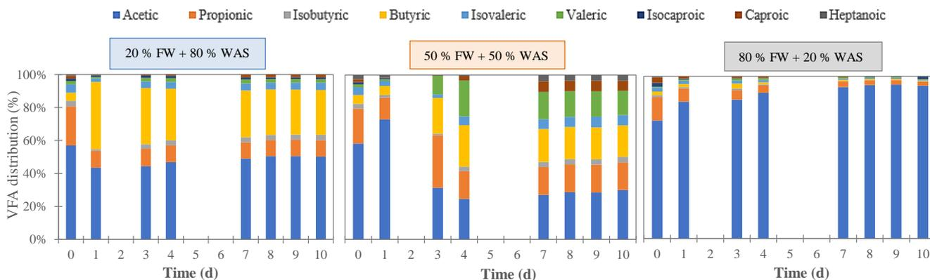
**Fig. 11** VFA distribution in different conditions when co-fermenting FW and pretreated WAS
