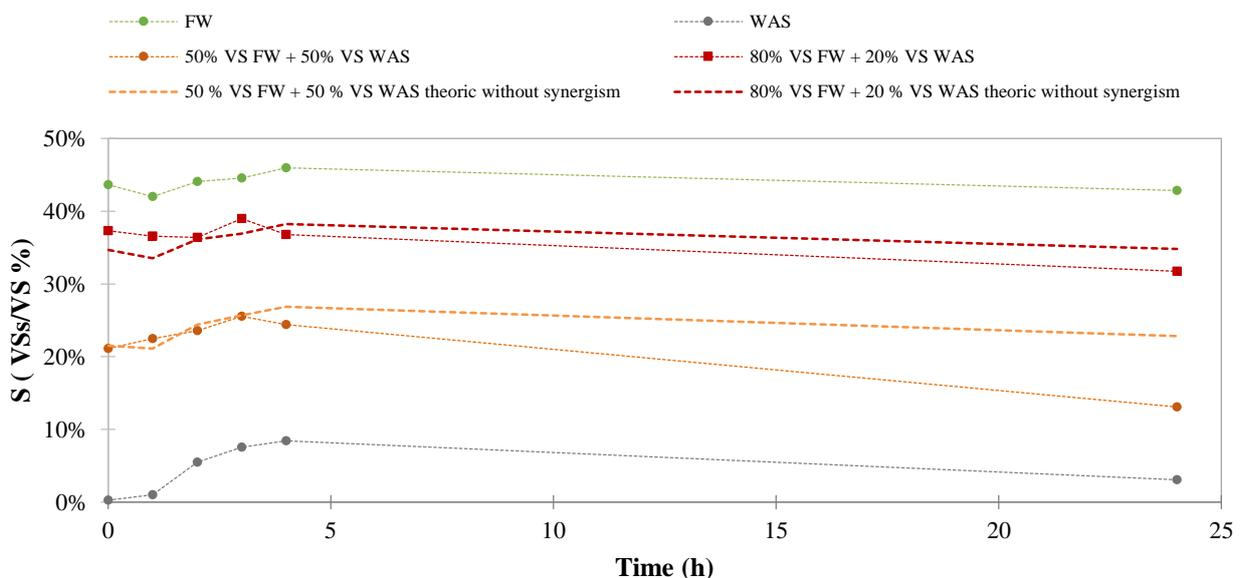
**Fig. 9** Change of solubilisation of FW with WAS under thermal pre-treatment at 55 °C during 1h 30 min (discontinuous curves are referred to the expected values of solubilisation if no synergism was observed)
