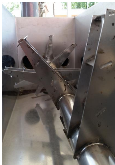
Figure 1: Detail of the pilot scale reactor agitation system
