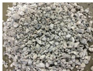
Figure 2. Coarse recycled concrete aggregates (CRCA).
