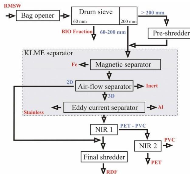
**Figure 1.** The designed mechanical – physical RMSW processing technology
