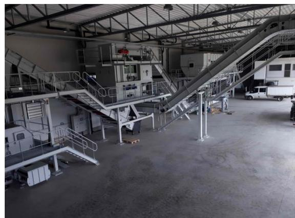
**Figure 3.** The drum sieve (back) and the KLME separator (front)
