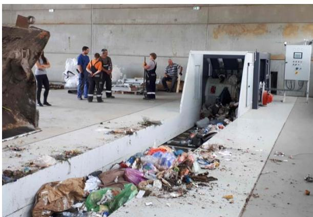
**Figure 2.** The moving floor conveyor and the bag opener
