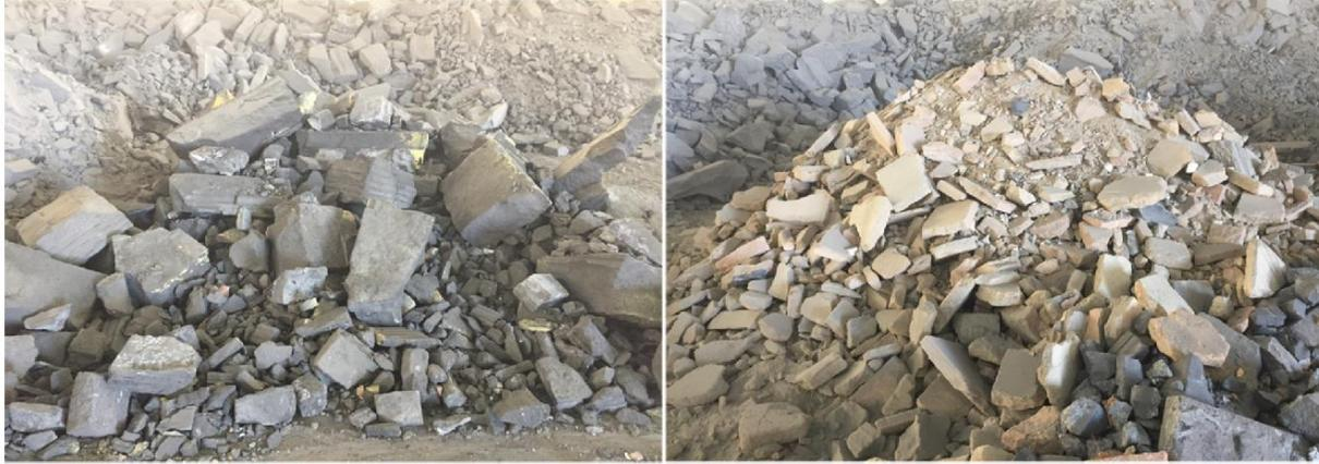
Fig. 1. 1<sup>st</sup> SPL cut of carbonaceous grade (left) and 2<sup>nd</sup> SPL cut made of refractory, insulation bricks, and ramming paste (right).
