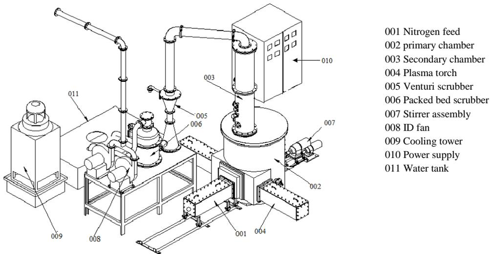
Fig.1. Schematic diagram of the plasma waste processing plant
