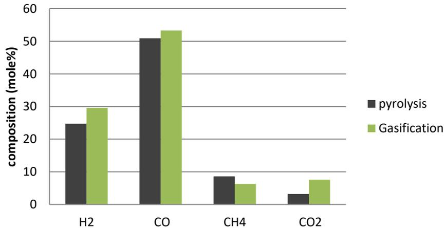
Fig.2. Gas composition of plasma pyrolysis and plasma gasification
