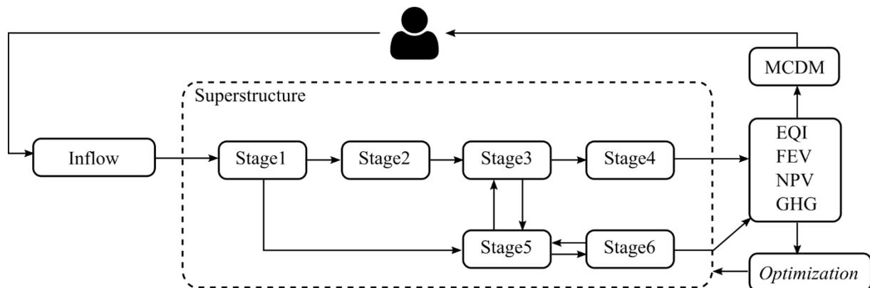
**Figure 1.** DSS framework for a WWTP superstructure with resource recovery units.
