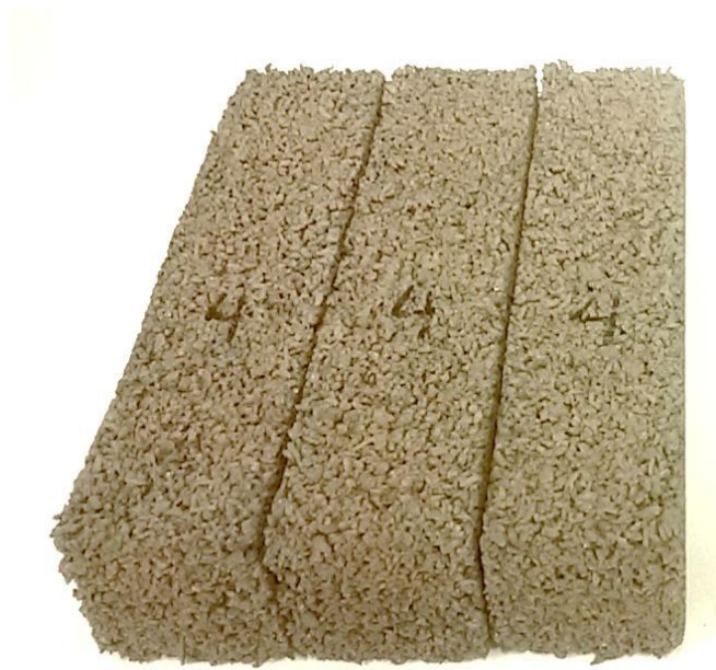
Figure 1. Digital photograph of the cork-containing alkali activated composites (4 cm x 4cm x 16 cm).
