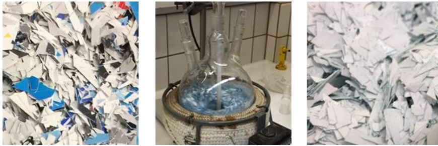
Figure 3: banner flakes before, during and after de-inking.
