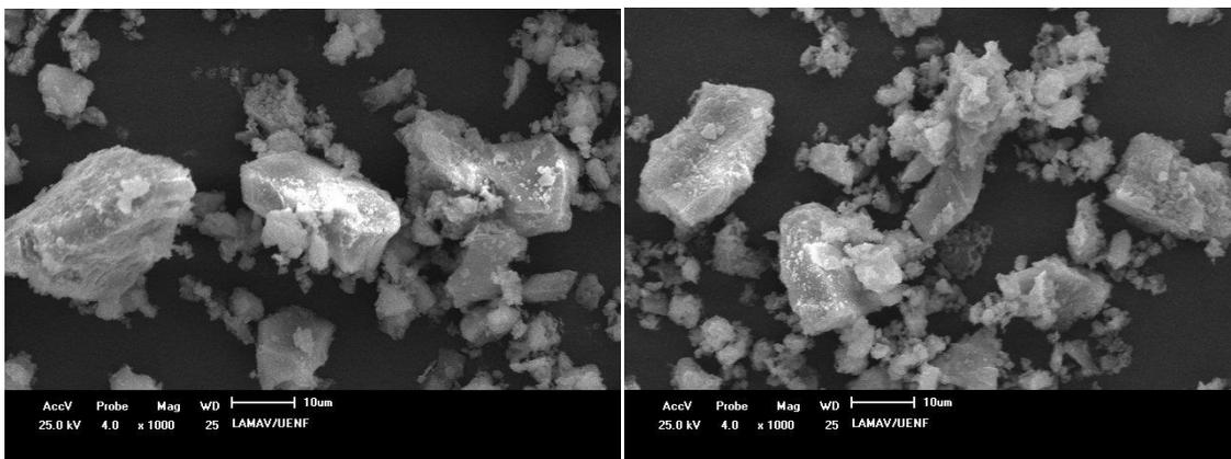
Fig. 3 Glass polishing sludge SEM.
