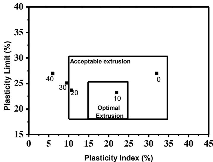
**Fig. 6** Extrusion prognosis of the formulations identified by the corresponding number of the quantity of waste incorporated.
