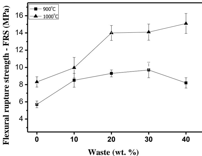
Fig. 9 Flexural rupture strength of the fired specimens as function of GPS incorporation
