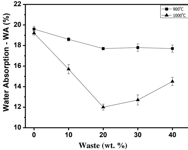
Fig. 7 Water absorption of the fired specimens as function of GPS incorporation.
