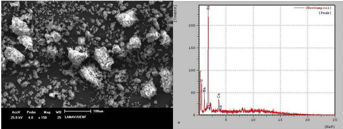
Fig. 4 Glass polishing sludge SEM with EDS.
