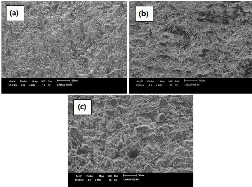
**Fig. 12** Scanning electron microscopy of the formulations containing 0, 20 and 40% of GPS fired at 1000 °C.
