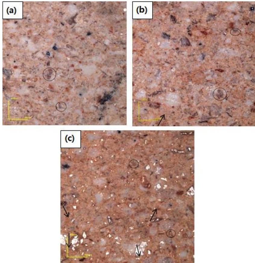
**Fig. 10** Optical microscopy of the formulations containing 0, 20 and 40% of GPS fired at 900°C.
