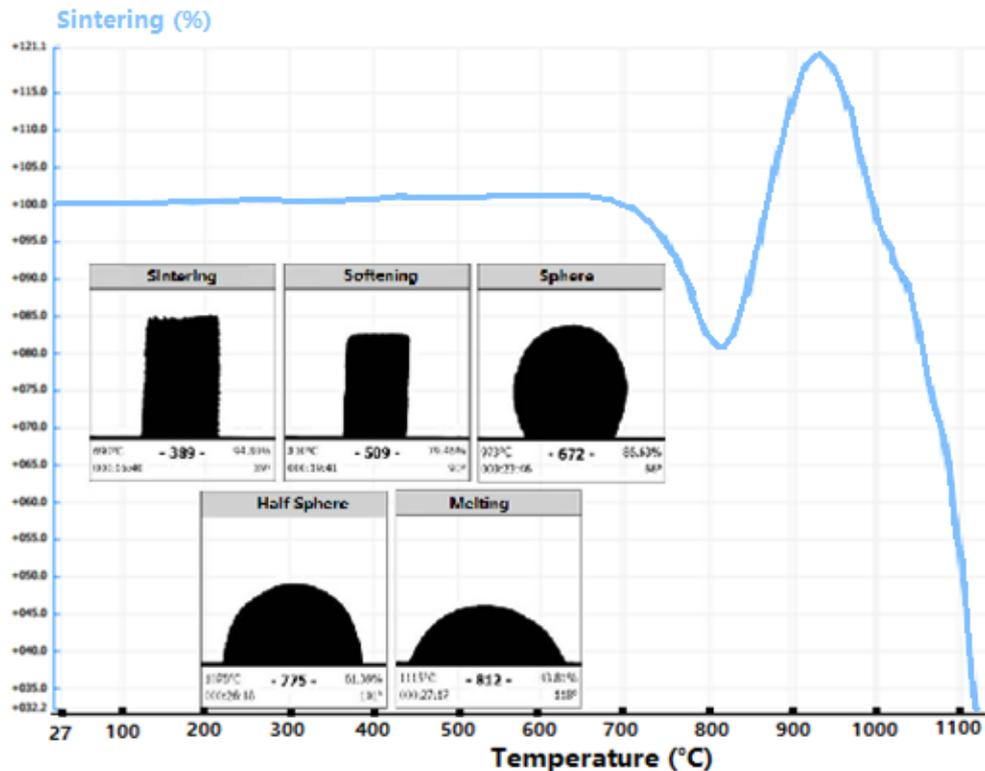
Fig. 5 Optical dilatometry of glass polishing sludge
