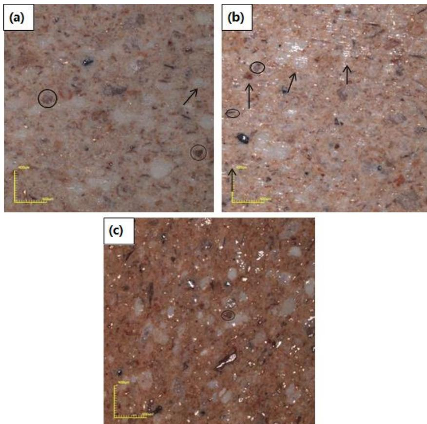
**Fig. 11** Optical microscopy of the formulations containing 0, 20 and 40% of GPS fired at 1000°C.
