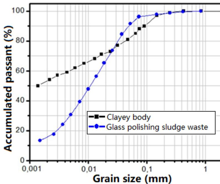
Fig. 2 Particle size distribution of the glass polishing sludge.
