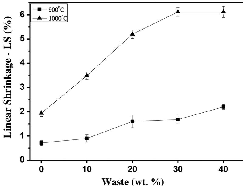
Fig. 8 Firing linear shrinkage of the fired specimens as function of GPS incorporation
