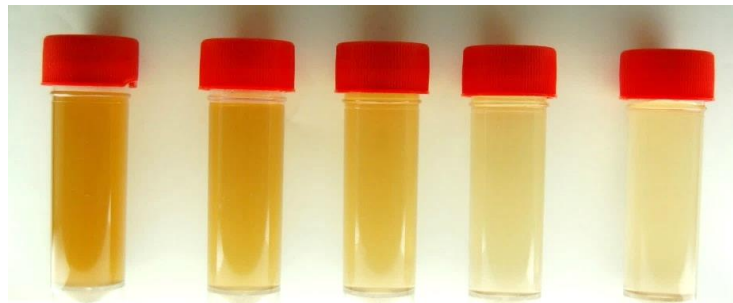
Figure 3. Samples obtained during the extraction of 10g of olive pulp using 100, 150, 200, 250 and 300 mL of water correspondingly (from left to the right).
