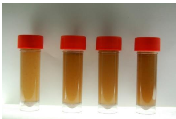
Figure 7. Samples obtained from the extraction of 20g of olive pulp using 200mL of distilled water at 150 rpm for stirring rates ranging between 50, 100, 150 and 200rpm correspondingly.
