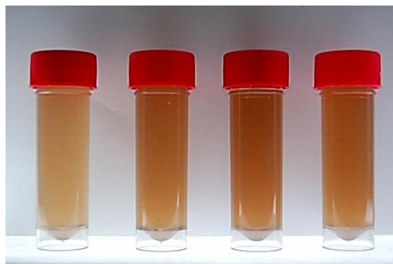
Figure 5. Extracted solutions obtained during the extraction of 20g of olive pulp in 200mL of water for stirring duration 15, 30, 45 and 60 minutes correspondingly.
