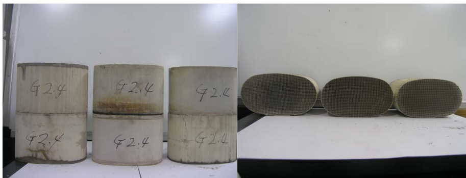
Figure 1. Images of spent auto-catalyst with honeycomb structure used in this study.
