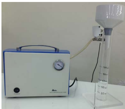
Figure 2 Time to filter (TTF) a certain volume test equipment
