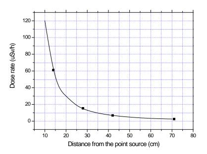
Figure 1. The acceptable dose rate at several distances from the point source. Analytical results are presented by the solid line and MCNP simulation results by the points.
