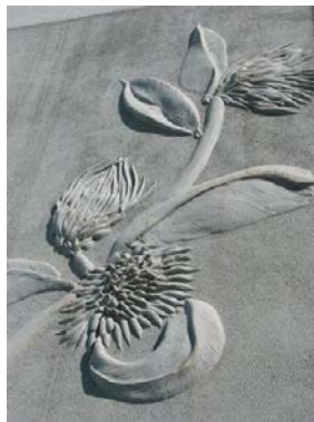
Figure 4. Surface made by SCC
