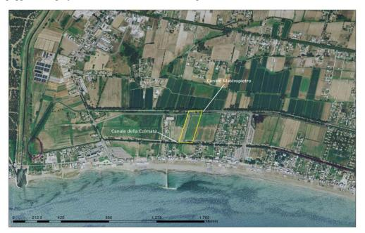
The project provides three phytoremediation systems, fed by water coming from the Colmata canal, with more polluting load, and re-entered, treated, in the Matropietro canal. At the end of the realization of phytoremediation system and of the green areas, a parking space, a dining area and pedestrian and cycle paths have also carried out.
