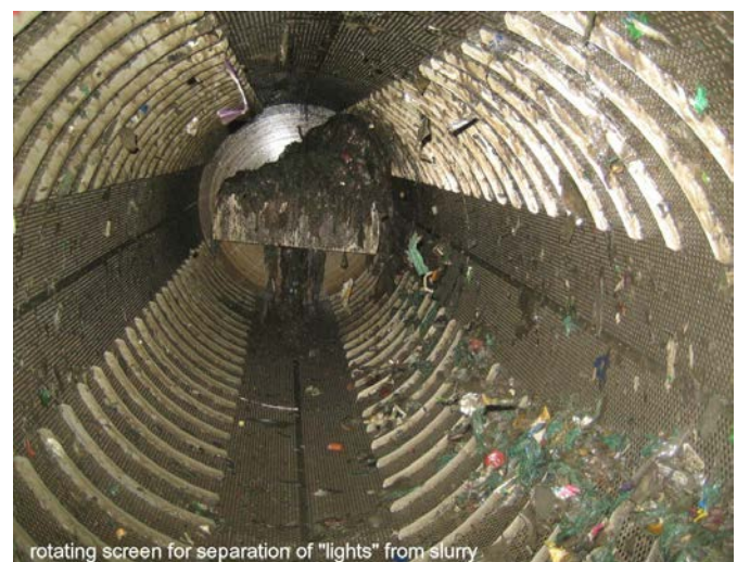
rotating screen for separation of "lights" from slurry
