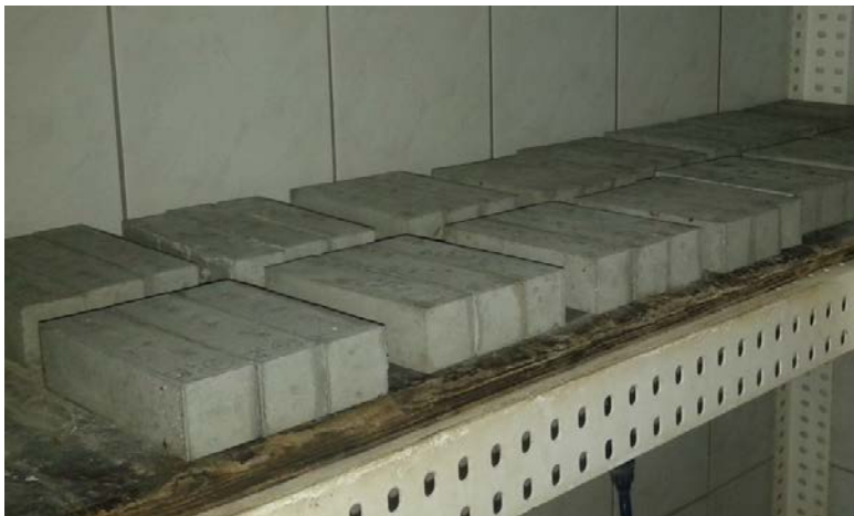
Fig. 5 Mortar specimens prepared for mechanical strength tests in the laboratory at the Faculty of Civil Engineering University of Zagreb
