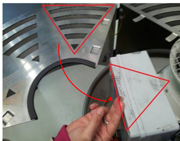
Fig.2 - Iron dust deposit at the top of the machinery, replicating the triangular shape of the protection grid
