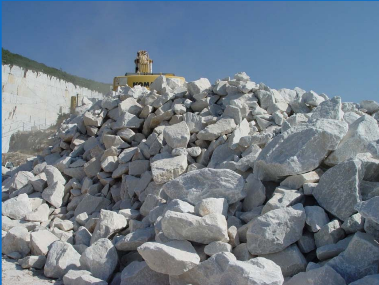
Marble waste prepared to feed a fillers producing mill (Stenopos)
