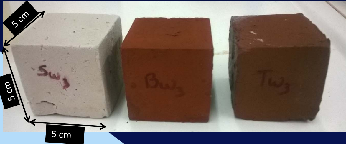
Geopolymers from concrete, bricks and tiles (left to right)
