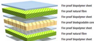
Fig. 1. Scheme of multi-layer sandwich panel to be developed within BRIGIT project
