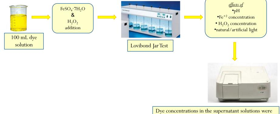
Dye concentrations in the supernatant solutions were measured by UV/Visible Spectrophotometer (V-530 Jasco UV/VIS)
