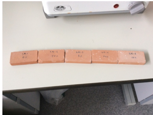
Figure 2 Sintered bricks. Marble sludge increases from left (0 wt%) to right (10 wt%)
