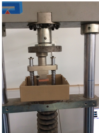
Figure 3 Application of the load during the compressive test on one specimen
