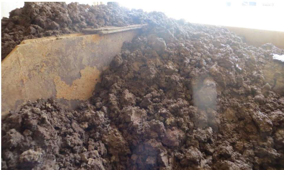
Figure 02 – Centrifuged sludge from WTP Porto das Caixas with solids content higher than 30%.
